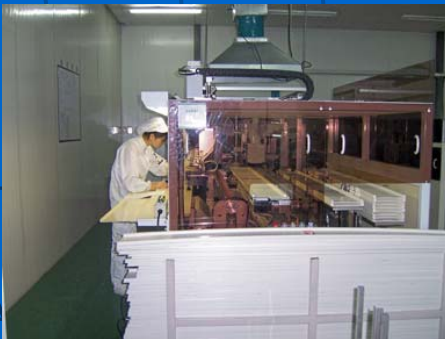
Automatic Cell Tabbing and stringing
